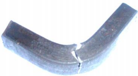
Fig. 1.4(a): Square bar cracks on
